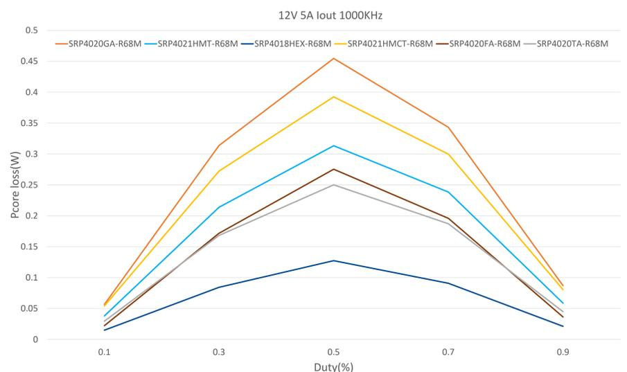
Fig. 7. Measured core loss of different inductors at different duty cycle when the operating frequency is 1000 kHz.
