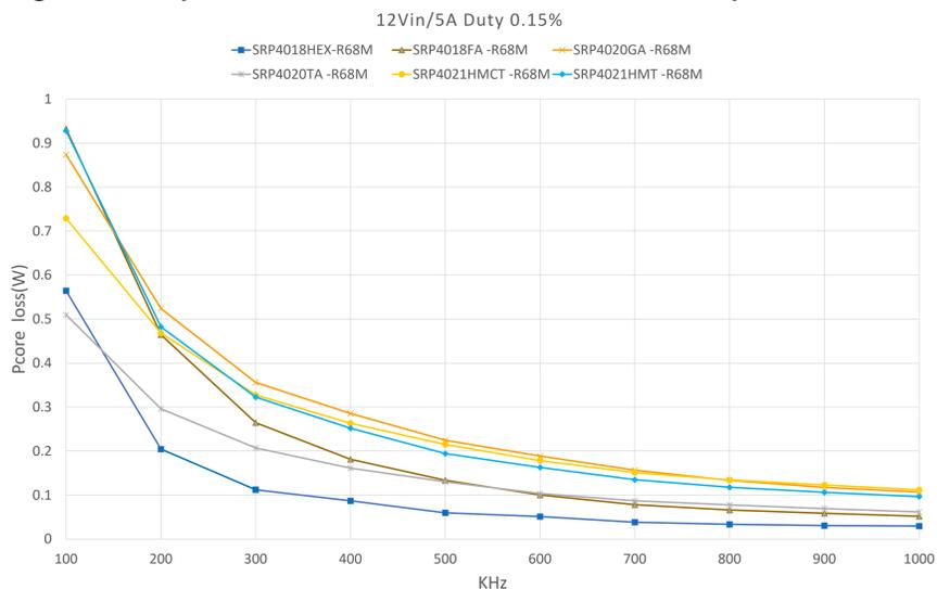
Fig.3 . Measured core loss at different operating frequencies when the peak-to-peak value of triangle current is 5 A from the MADMIX tester.
