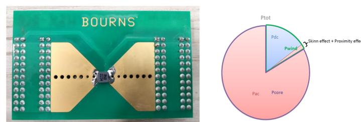
Figure 2.1: DUT sample and Power loss definitions (Pac+Pdc=Ptotal loss=Pcore+Pwind).
