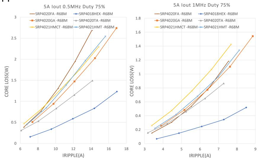
Fig. 5 Fig. 6. Measured core loss of different inductors at different I ripple values when the operating frequency are 500kHz & 1000 kHz.
