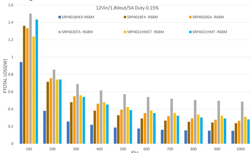
Fig. 4. Measured total loss at different operating frequencies when the peak-to-peak value of triangle current is 5 A from the MADMIX tester.
