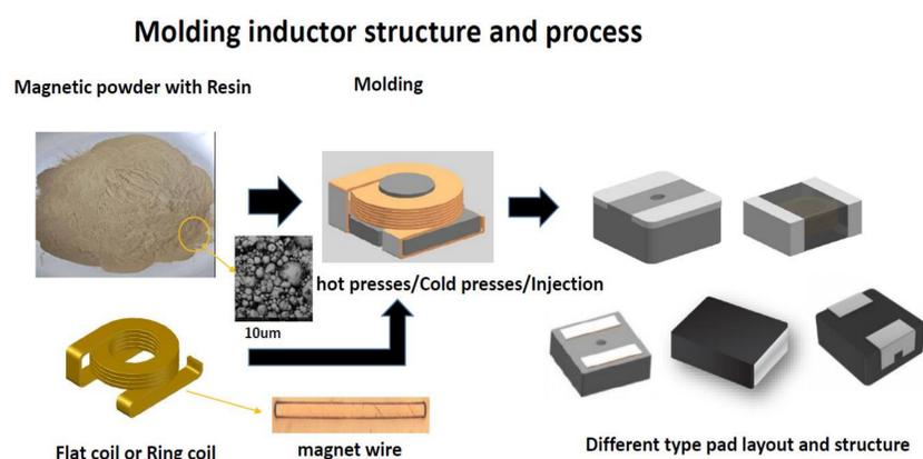
Fig. 1. Molding process
